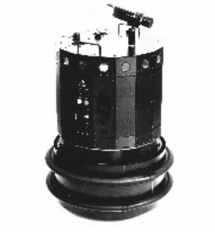
Fig. 1. Fortytwo , the Nomad 200 robot used in the experiments. The robot is equipped with 16 sonar and 16 infrared sensors, flux gate compass and an odometry system. The camera visible in the photograph was not used in the experiments presented here.
